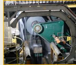
The Castrip process utilizes the concept of twin-roll strip casting and represents the first commercial installation of direct casting of carbon steel sheet products. Among the main advantages of this new technology is the fact that the steel is cast at or near its final thickness. This eliminates the need for large hot and cold rolled reductions and provides unique product properties.
