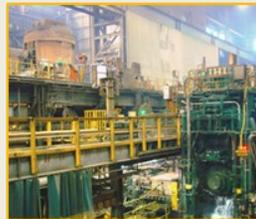
Constructed in 2001 and commissioned in 2002, the Castrip facility is capable of producing 500,000 tons annually. Located at Nucor's Crawfordsville Indiana steelmaking site, Castrip UCS (Ultra-thin Cast Strip) products are sold as hot rolled, cold rolled and galvanized sheet. The product conforms to ASTM standards A1011, A1039 and A658. Typical applications for UCS products include structural decking,
