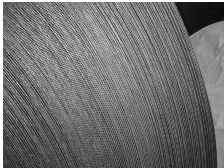
Fig. 8 - Photograph of an untrimmed, as-cast UCS coil edge.
