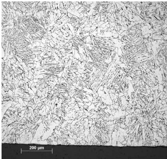
Fig. 7 - Typical as-cast UCS microstructure indicating a mixture of polygonal and acicular ferrite.
