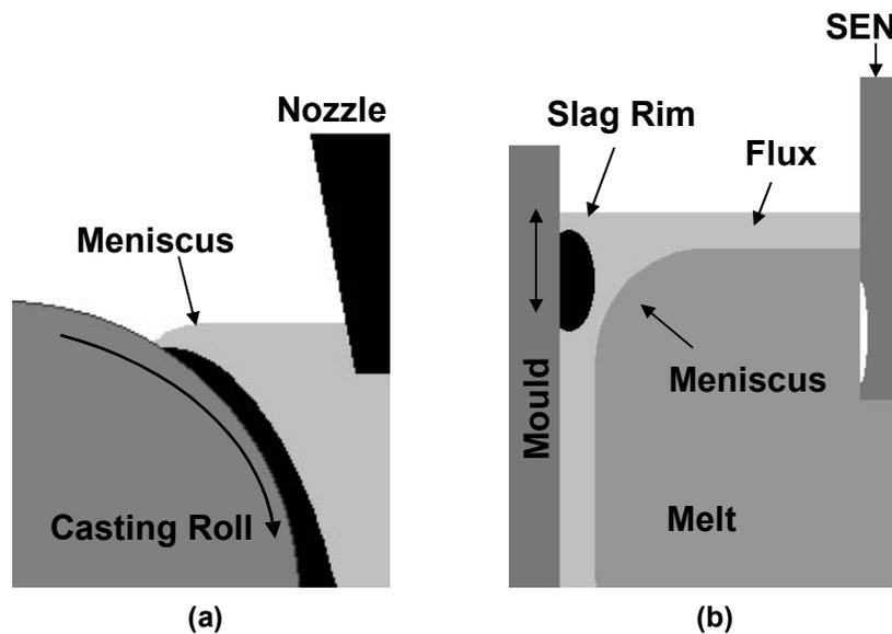
Fig. 2 – Comparison of the meniscus region in (a) the CASTRIP process and (b) conventional slab casting.
