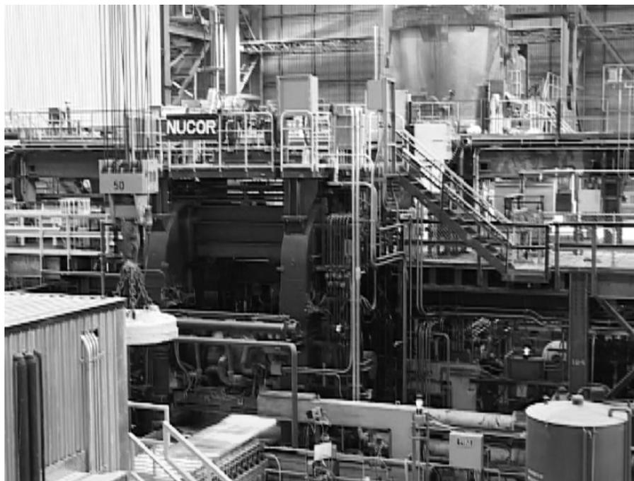
Fig. 7 – Photograph of Nucor’s CASTRIP plant during commissioning. Note steel strip emerging from the single hot rolling stand.
