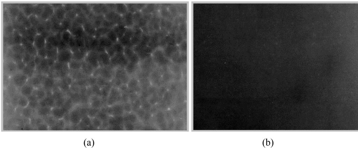
Fig. 3 – X-ray maps indicating the level of porosity in the solidified steel strip, (a) early casts showing porosity and (b) later casts with no porosity.
