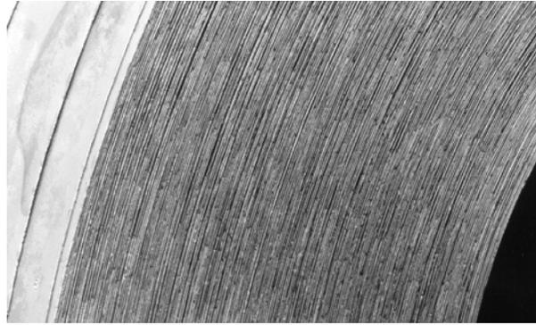
Fig. 4 – Photograph of typical coil sidewall produced with the Castrip process at Project ‘M’.
