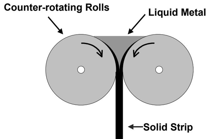
Fig. 1 – Simple schematic of twin-roll strip casting process.
