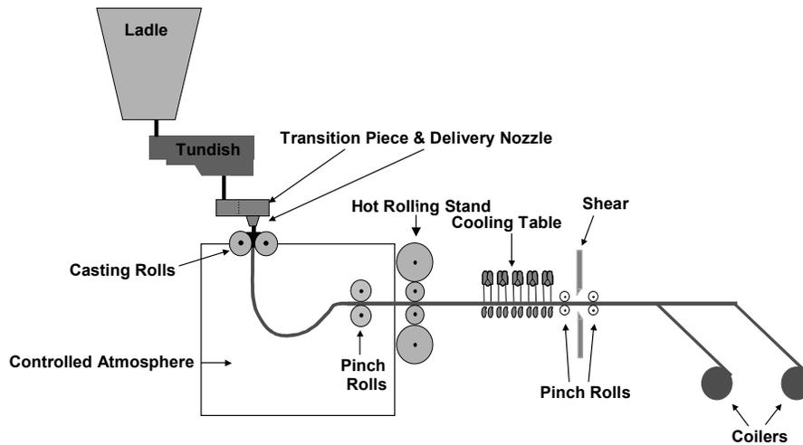
Fig. 6 – CASTRIP process schematic.
