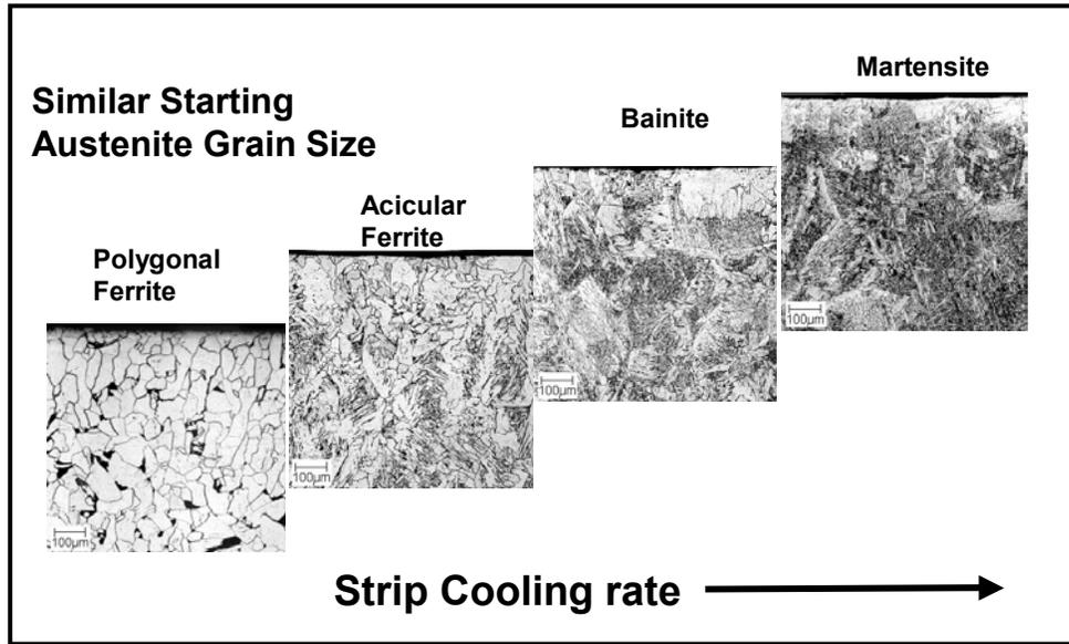
Figure 3 – Relative effect of cooling rate on the final microstructure of Castrip steel products
