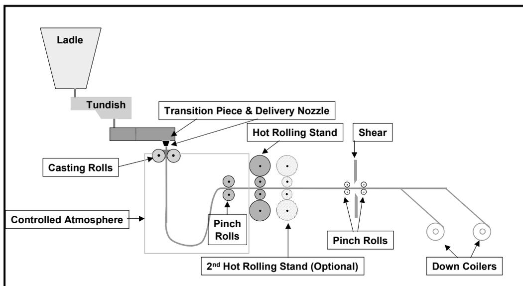
Figure 2 – Process schematic for Project ‘C’ plant layout
