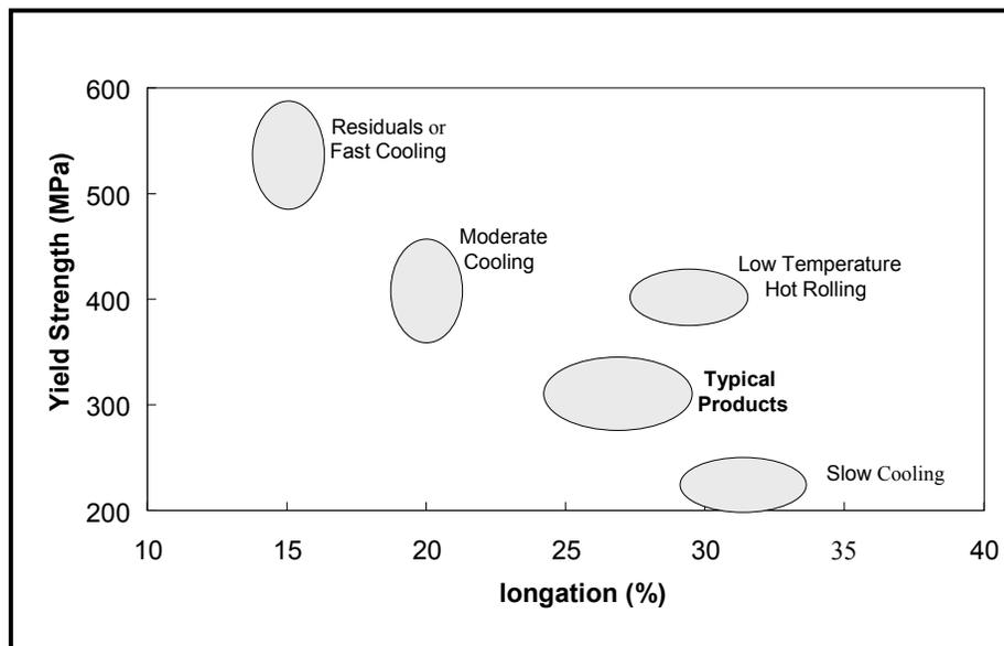
Figure 4 – Effect of cooling rate on the mechanical properties of CASTRIP strip products
