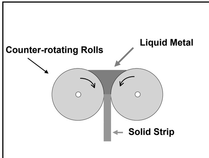
Figure 1 – Simple schematic of twin-roll strip casting process.
