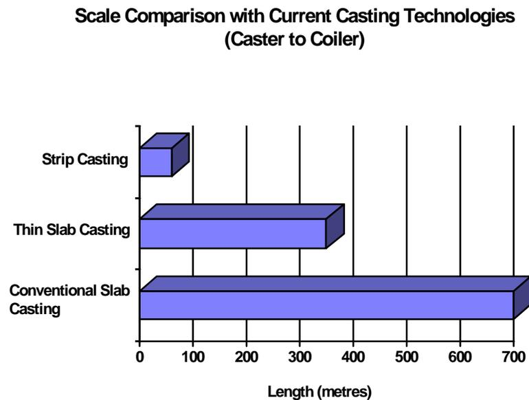
Figure 5. Line length from caster to coiler for various strip production routes.
