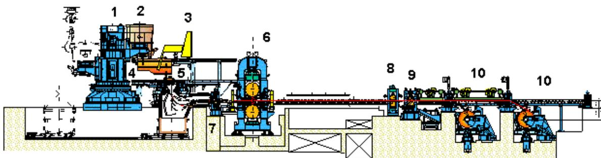
Figure 1. General arrangement of the development plant at Port Kembla. Main features: 1. Ladle Turret, 2. Ladle, 3. Plasma Torch, 4. Tundish, 5. Twin Casting Rolls, 6. In-line Rolling Mill, 7. & 8. Pinch Rolls, 9. Shear, 10. Coilers.
