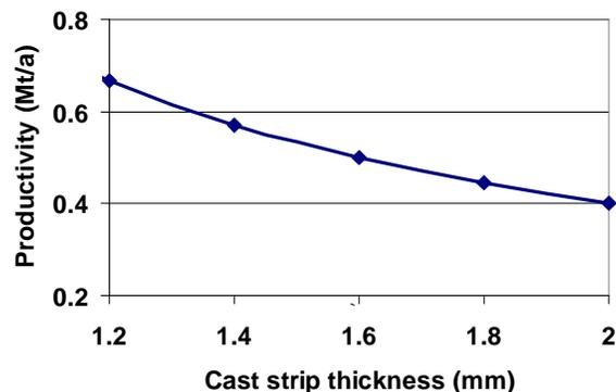
Figure 4. Effect of cast strip thickness on machine throughput (1233 mm wide, k-factor = 16.25, Yield = 94.1%).
