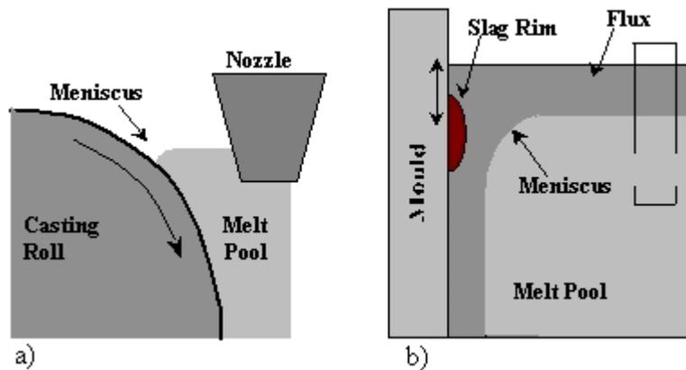
Figure 3. Schematic representation of moulds (a) twin roll strip casting (b) slab casting.
