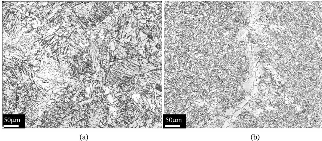
Figure 13. Optical micrograph of (a) Nb microalloyed UCS Grade 380 and (b) standard UCS Grade 380. (200X, Nital etch)
