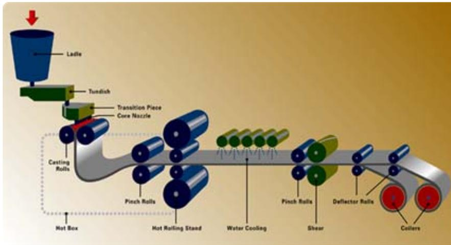
Figure 1. Main components of the CASTRIP process.
