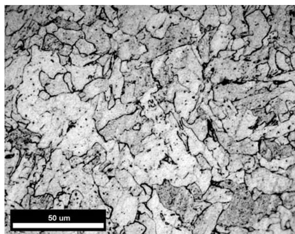
**Figure 1.** Light optical micrograph of low C Mn-Si UCS steel.
