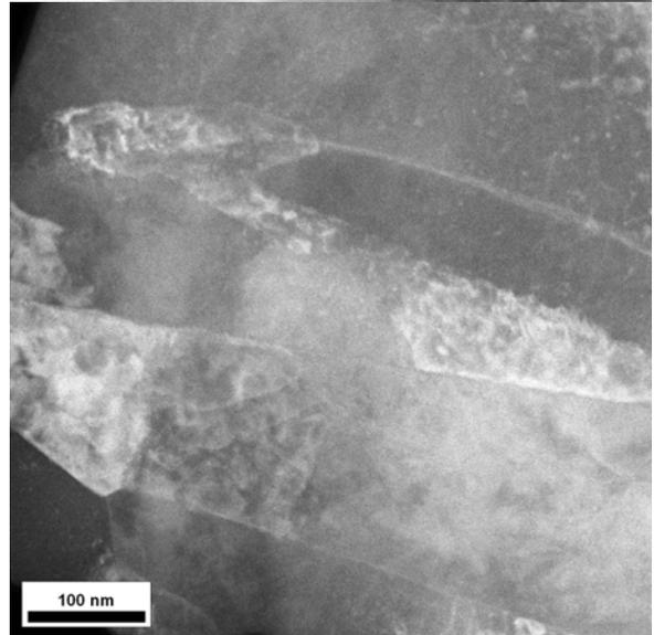
**Figure 4.** Bright field-dark field TEM micrograph of microalloyed UCS steel with 0.026% Nb.
