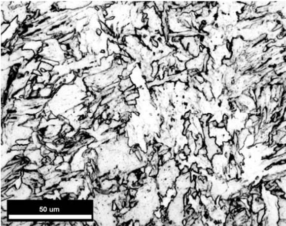
**Figure 2.** Light optical micrograph of microalloyed UCS steel with 0.026% Nb.
